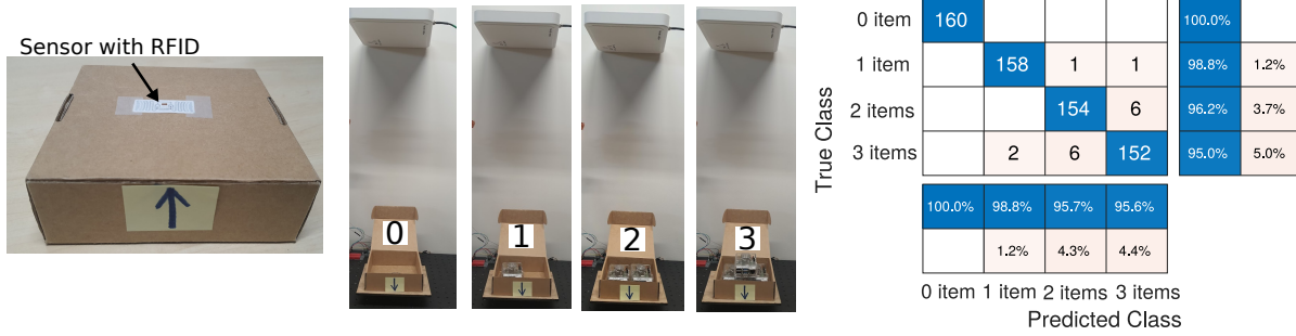
Fig. 19. Weighing objects placed in a box with ForceSticker RFID sticker stuck to the bottom of the package: By measuring the weight of the contents, ForceSticker is able to classify the number of contents in the box
